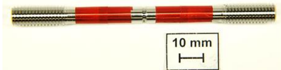
Figure 1: Round notched tensile specimen with self-adhesive galvanic tape prior to the test
